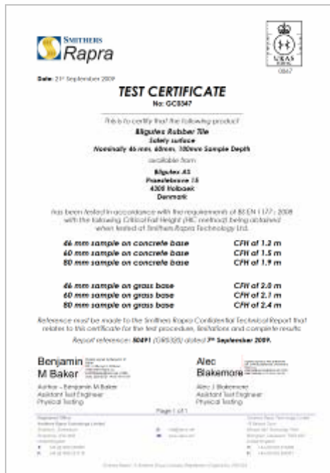
TEST CERTIFICATE No. GC0347 Playground tiles 46, 60, 80 mm Issued on: 21 September 2009 Issued by: Smithers Rapra, UK
